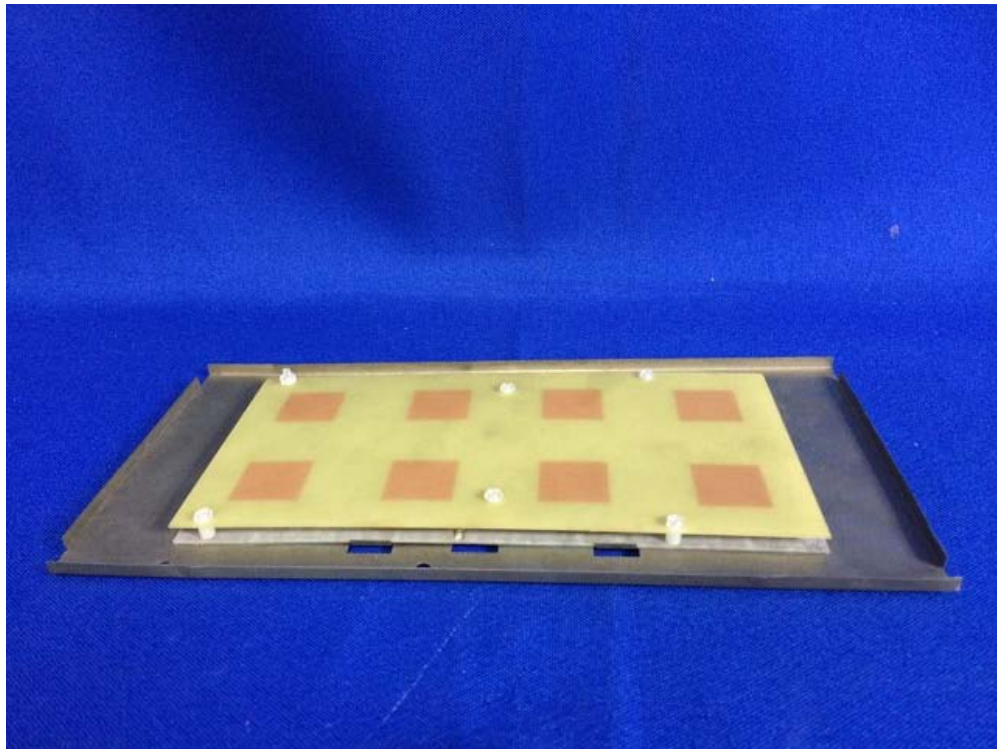
(15) EUT Photo (Panel Antenna 17dBi)
