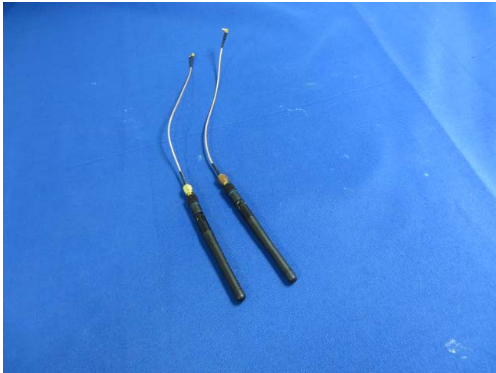
(5) EUT Photo (Dipole Antenna 2dBi)
